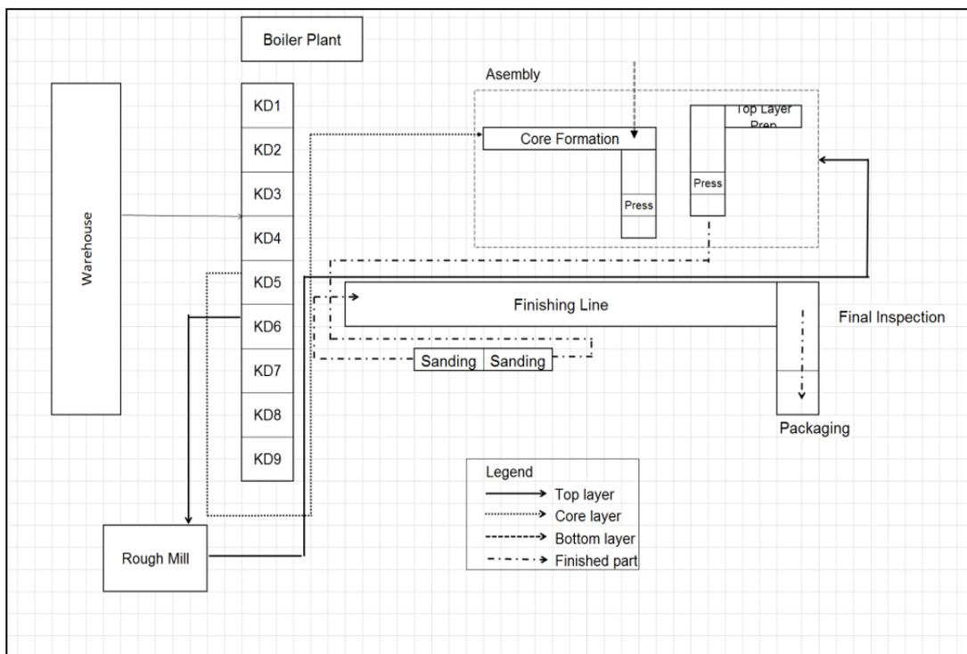
**Figure 1.** Existing layout (material flow)
