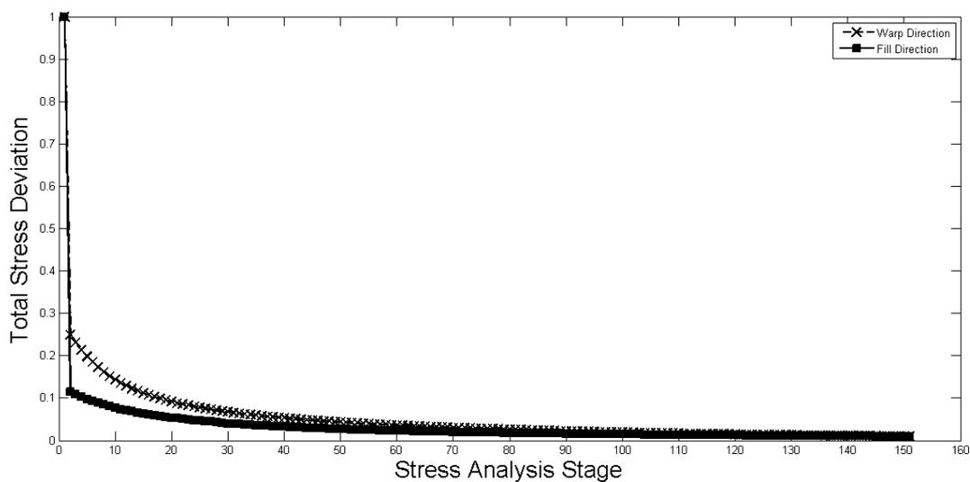
**Figure 8.** Convergent curve of Cable Reinforced Handkerchief Surface,  $u=v=0.6$
