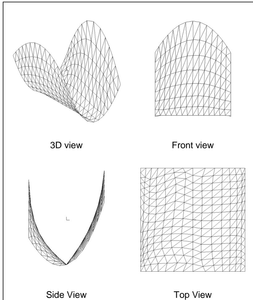
**Figure 7.** Initial Equilibrium Shape Cable Reinforced Handkerchief Surface,  $u=v=0.6$
